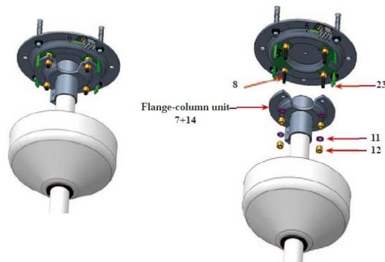
**N.** Screw (without locking) the nuts (12) and the remaining washers (11) on the screws (8) of the ceiling flange (1)
