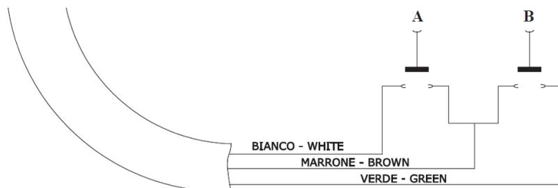
**3.2.3 Complete dental light connection to the ceiling, wall or floor (permanent)**
