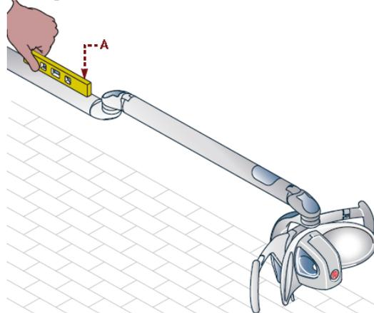
Connect the power supply cable according to the specifications outlined in Tab. 1. Check the light stays balanced in all positions. If necessary, use the adjustment system on the spring to balance the light.
