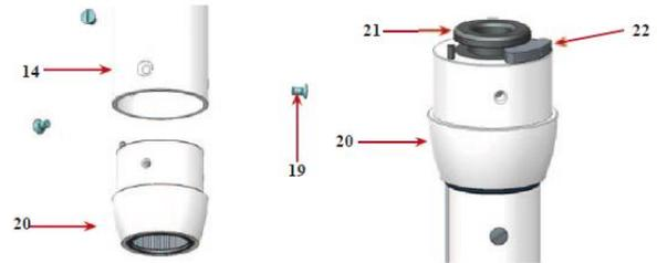
**R.** Slip - from the top - inside the column (14) a traction cord.
